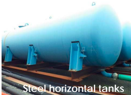
Steel cylindrical tanks (welded)
