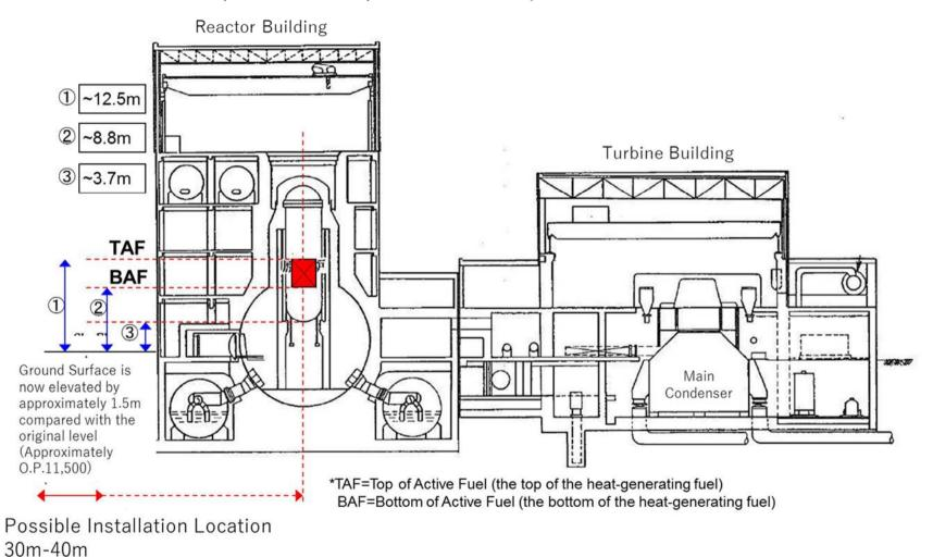
3. Location of Equipment Installation for Demonstration Test in No. 2 Reactor at Fukushima Daiichi NPS (Cross Section) \*Plan as of the present
