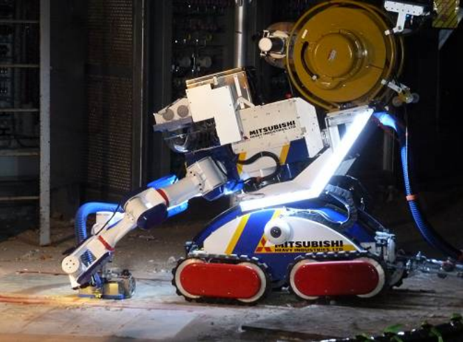
Suction/blast decontamination equipment
