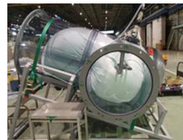
Fig.4 Auxiliary material test condition for closure of water stoppage of PCV bottom section
