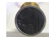
Fig.6 Water stoppage test status for water stoppage for PCV upper section
