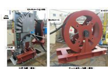
Fig.5 test device for water stoppage of PCV upper section
