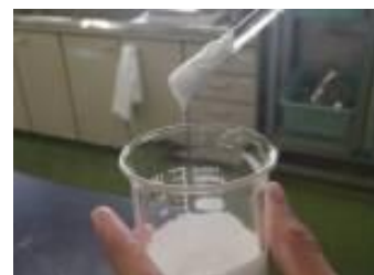
Fig.2 Sample of prototype of insoluble neutron absorber (gadolinia/slurry)
