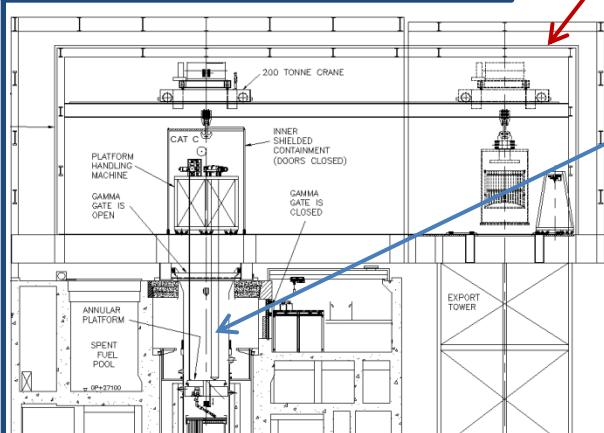
We propose the use of shielded containment structures and a ventilation system to contain radiation and contamination. A top down system using a suspended work platform is deployed for access into RPV.
