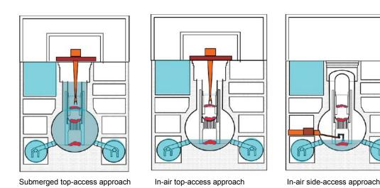
Source: "Plan of technical strategy for decommissioning of TEPCO's Fukushima Daiichi Nuclear Power Station - toward Mid-and-Long-Term Roadmap 2015" by the Nuclear Damage Compensation Facilitation Corporation (NDF), April 30, 2015 Figure 1: Outline of approaches of fuel debris retrieval
