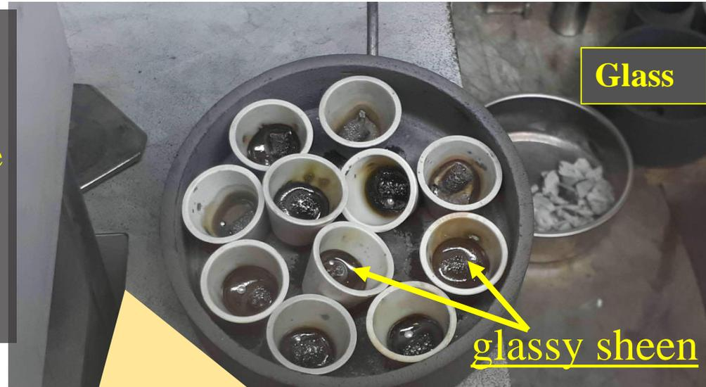
In three crucibles, the metallic phase samples with curium did not dissolve completely, possibly due to the difference in the composition of the concrete loaded into each crucible (the amount of rubble in the concrete in different crucibles was not the same).
