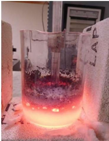
Condition of Quartz Beaker Removed After Heating (Melt 5 Material)
