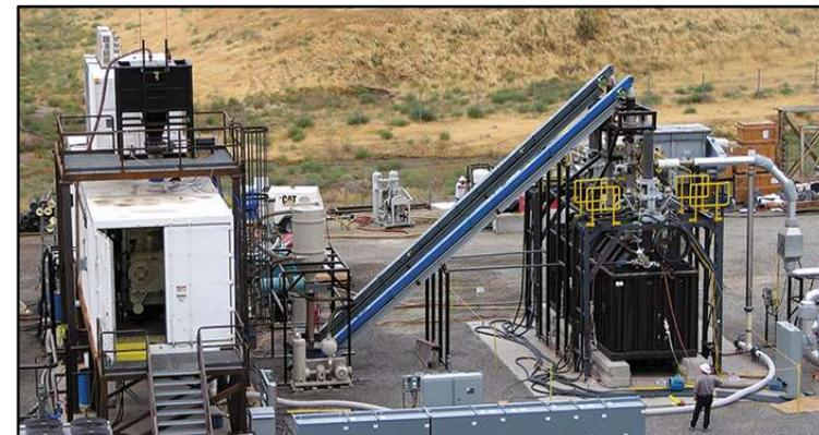
**GeoMelt® ICV™ – Hanford Demonstration Bulk Vitrification System (DBVS): 50 ton Melts, USA**
