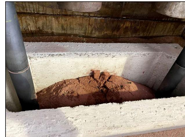
*View into the melter showing surface of simulated failed melt. The material visible is not glass because the melt was suspended before completion according to the test plan*
