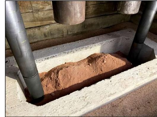
*Looking into the melter showing 80 kg of test materials, feed pipes, electrodes, and refractory*
