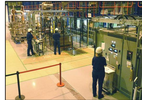
**GeoMelt® ICV™ – Radioactive Test Rig Sellafield Site: 500 kg Melts, U.K.**
