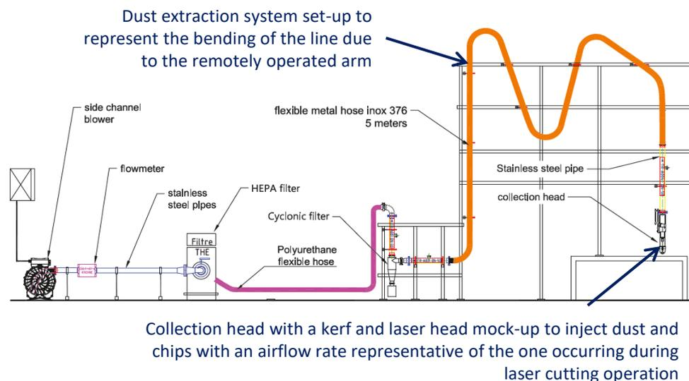
Transportation efficiency tests have been done with alumina powder (①), titanium and iron (②) granules and chips of zirconia coming from previous laser cuts (③). The transportation tests concern the first part of the dust extraction system from the collection head to the cyclonic filter in which particles are recovered (in orange in the figure of the right, flexible hoses are made in stainless steel). The transportation efficiency goes from 95 % to 100 % depending on the particles.
