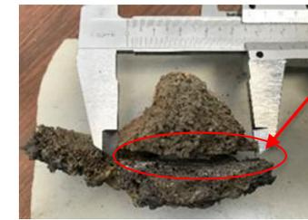
Measurement of material mass loss during cutting n° 6 on the Fuel Debris sample
