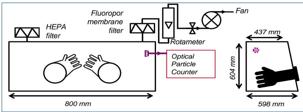
TRANSAT is a small glove box (250L). This facility is instrumented with an optical particle counter (GRIMM, size range 0,25 µm – 30 µm)
