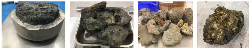
The total mass of in-vessel fuel debris simulant blocks produced is 35 kg. Various shapes have been obtained (4 melting procedures)
