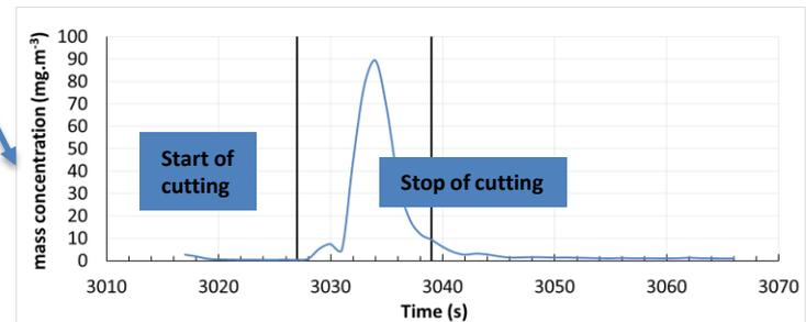
Measurement of mass concentration integrated through the cutting time with measured airflow
