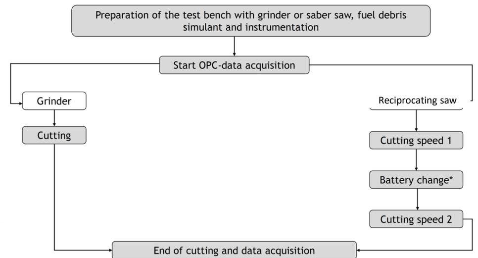
Operations are realized manually (no automation of devices). Therefore, cutting strenght has not been monitored and can have variations due to the operator.
