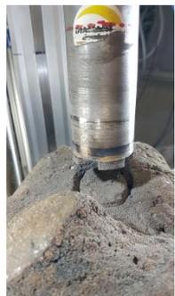
Core boring test of ex-vessel fuel debris simulant. Bore coring appears to be difficult, even impossible, when the tool cuts into melted and compact metal cluster. Also, cutting tool is quickly damaged and needs to be changed frequently
