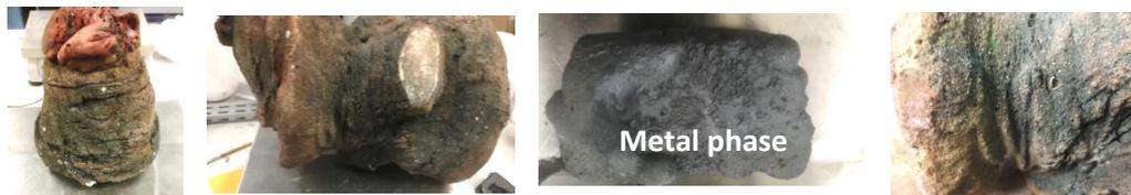
The total mass of ex-vessel fuel debris simulant blocks is 38 kg (including blocks of denser solidified metal) (4 melting procedures)
