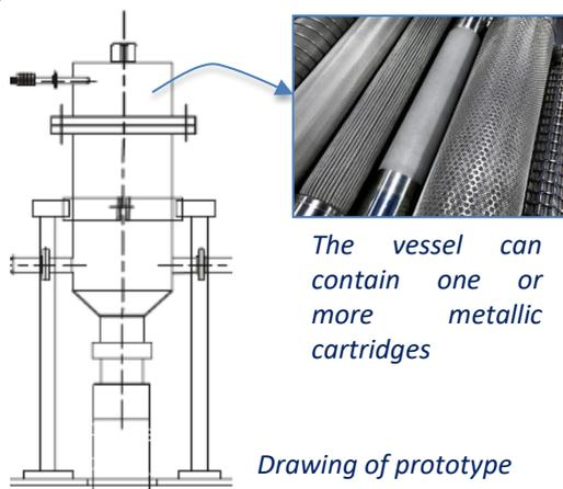
In order to optimize the design of the filter, preliminary tests have been conducted in lab facility on samples. These samples were different stainless steel grid that can compose the cartridge.
