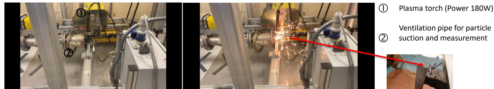
Particle number concentration during successive cutting/heating with plasma torch
