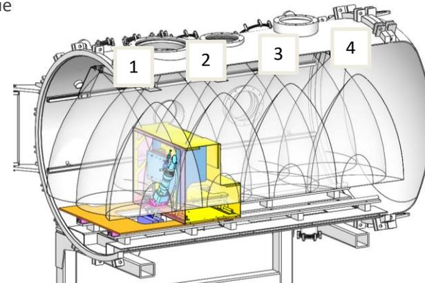
View of DELIA facility. The bottom figure shows the implementation of the laser cutting head and the 12 spraying nozzles (4 ramps of 3 nozzles). It is possible to use 1 to 12 spraying nozzles
