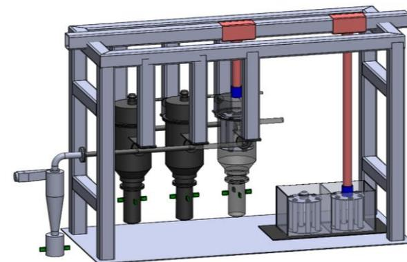
Dust filtered by the cyclonic filter and self-cleaning system and full cartridges of fine filtration system can be put into cans designed to be **compatible with unit cans and storage canisters**.
