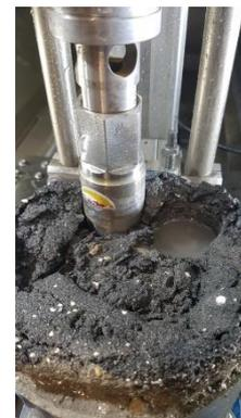
Core boring test on ex-vessel fuel debris simulant with spraying system on
