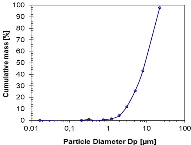
Figure on the left shows the cumulative mass of observed particles depending their diameter
