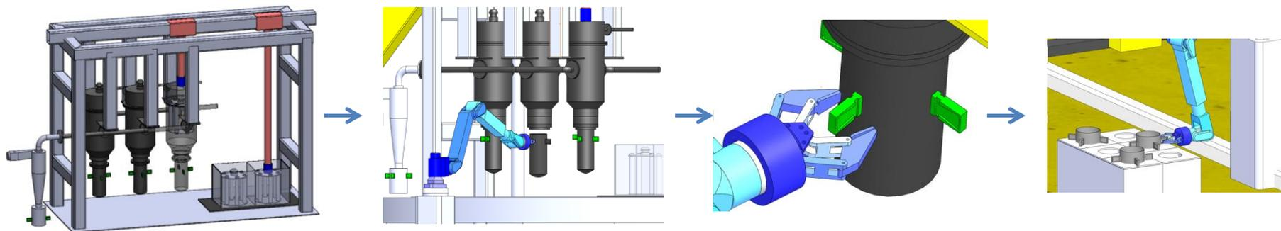
Tools (cutting tools, collection heads, suction tools) are disposed in a rack. Compatibility with existing cutting scenarios was checked.
