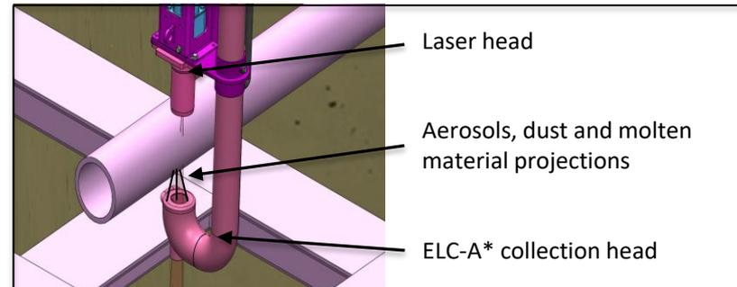
Illustration: cutting an element (with or without fuel debris) creates not only aerosols but also molten material projections
