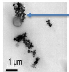
Aggregates of very fine particles (fractal like for laser cutting)
