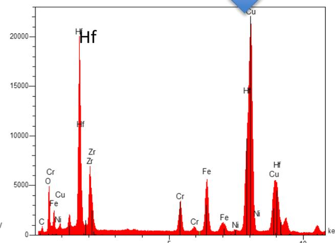
No nitriding reactions were characterized with EDS. Oxidation reaction are amplified for N<sub>2</sub> + humidity cutting
