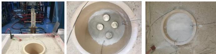
Crucible is filled with pellets and raw materials before melting
