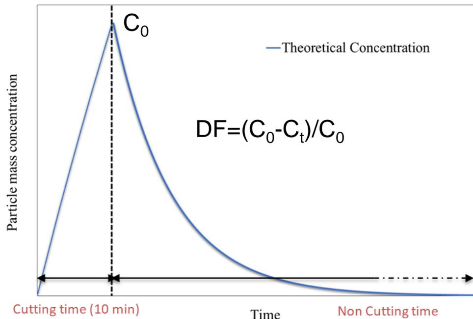
For this scenario, a cutting time of 10 min is considered and the non cutting time has to be evaluated depending of the concentration time evolution or Decontamination Factor (DF)
