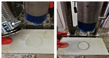
The cast fused Zirconia block is almost clean after the trial with extraction (on the left), which is not the case without extraction (on the right).
