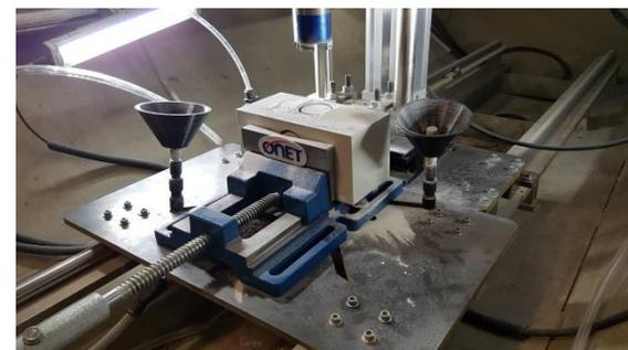
Core boring test on a cast fused Zirconia block. The core boring produces a very thin powder
