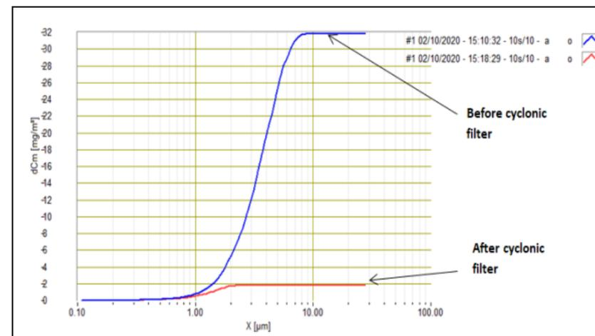
Example of mass concentration measurements before and after the cyclonic filter with polydispersed aerosols with different mean aerodynamical diameters (3.1  $\mu\text{m}$  and 4.7  $\mu\text{m}$ )
