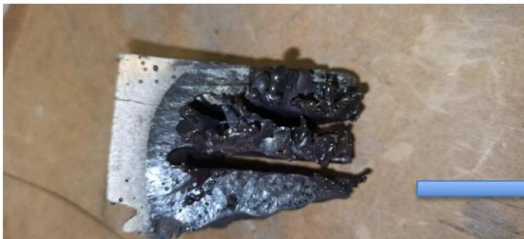
Laser cutting tests have been performed on the same sample of ex-vessel fuel debris simulant in dry conditions with air and then with nitrogen.
