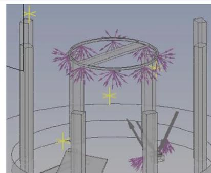
1 spray bar with 8 nozzles and large angle: it represents a global spray configuration, covering of large area at the bottom of the pedestal
