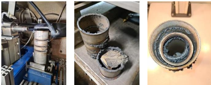
All configurations gave high collection efficiency rates (above  $\approx 93\%$  when considering number concentrations and around  $85\%$  when considering mass concentrations). Coating of collection head proved to be efficient during these tests (few deposition that is easy to remove).
