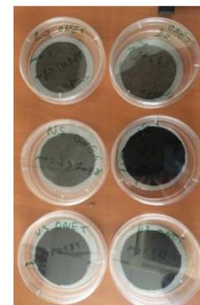
Two compositions of cartridges (number of layers and type of mesh) have been determined to be promising following these tests (Configuration 1 with 2 layers of very thin mesh and Configuration 2 with 1 layer of ME mesh and 1 very thin mesh)
