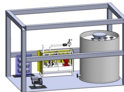
Water tank and spray scrubbing equipment rack
