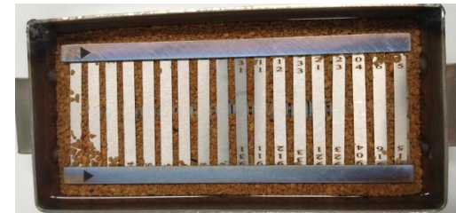
An overall view of the samples. T = 25 °C, t = 3000 h, [Cl - ] = 100 ppm. Without radiation
