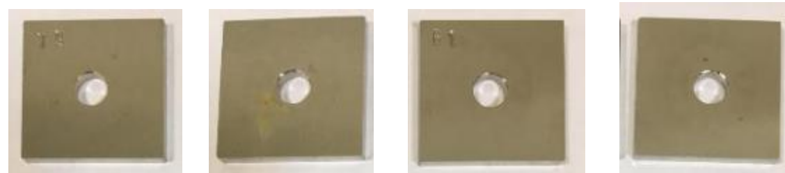
The overall view of the samples tested under the following conditions: [\text{Cl}^-] = 10 ppm, T = 60^\circ\text{C}
