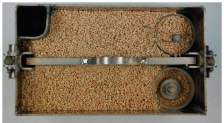
Container filling with Zeolite
