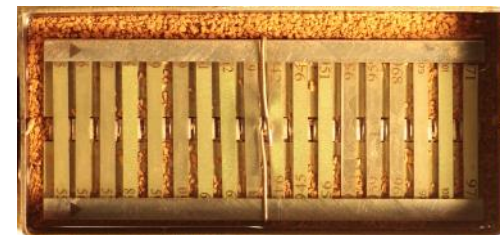
An overall view of the samples. T = 25 °C, t = 3000 h, [Cl - ] = 100 ppm. With radiation
