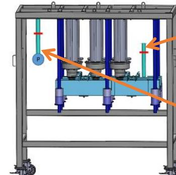
✓ Test ID 11 : Cutting of an ICM (In Core Monitor) tube (Solid rod, 56 mm diameter) with laser at 150 mm distance.
