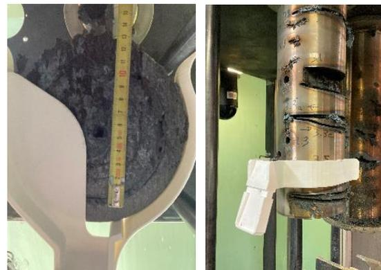
Plate fall prevention system in place in the CRD-H
