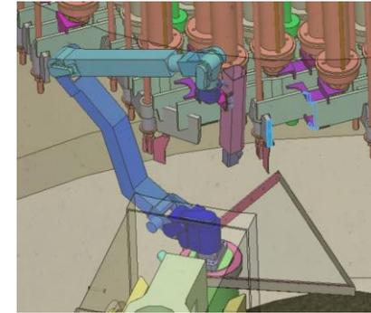
Cutting the support bar with the curved laser tool on the arm and the recovery platform on the carrier
