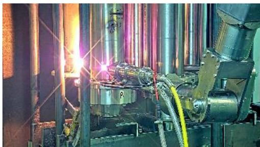
Cutting of CRD-H configuration A with flange
