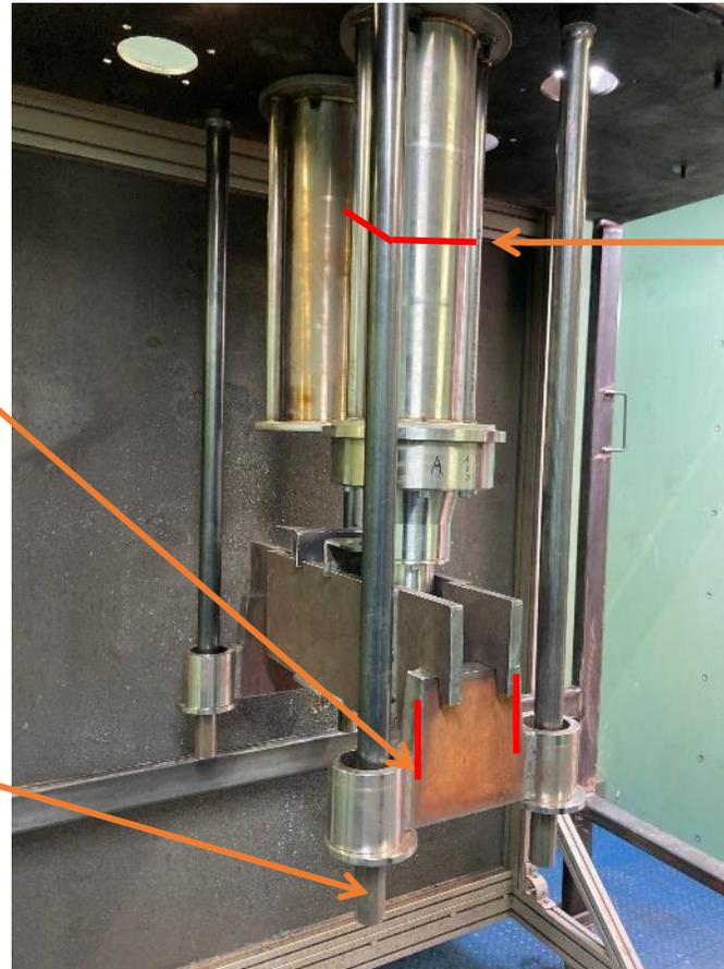
Configuration 2 of the bottom vessel CRD-H mock-up
