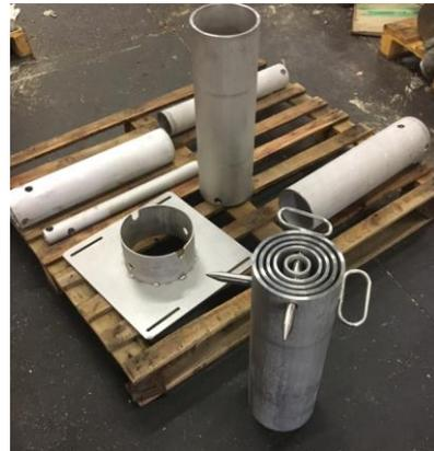
Picture of the mock-up of CRD-H for performance assessment of cutting tools
