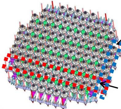
Row: set of CRD-H located perpendicular to the GRID supports between two rows of tie rods,
