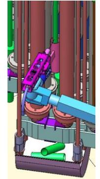
Cutting of the ICM with the cylindrical bucket on the arm
