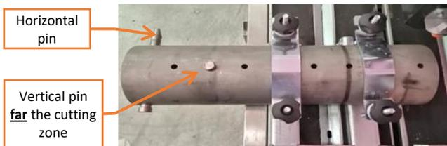
➡ High vibration and blocking the disk at the end of the cutting process
