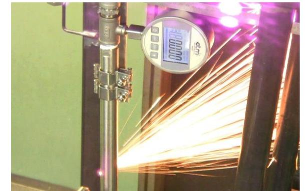
HCU filled with water and instrumented during cutting
