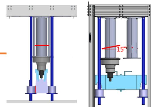
✓ Test ID 10 : Cutting with a 15° angle a CRD-H (configuration A)
