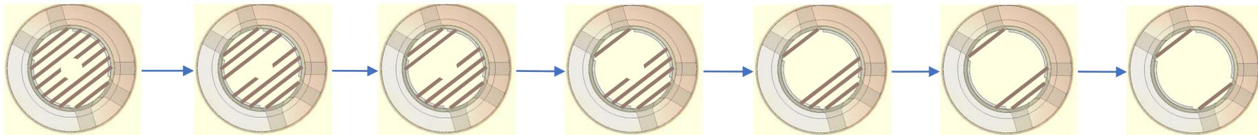
**Second situation:** central beams are damaged, therefore, the dismantling starts in the middle. Two beams remain at the end
