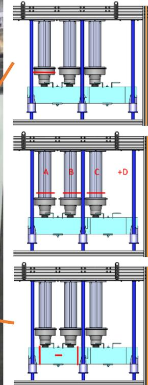
✓ Test ID 5 : Cutting of the CRD-H just above the top of the flange
