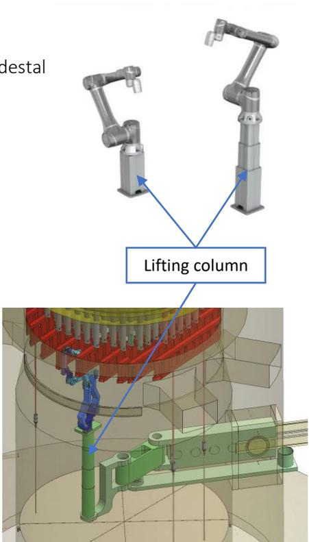
In order to reach the top elements of the pedestal, a lifting column is necessary on the carrier.
