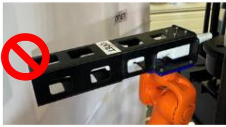
In red are presented the elements not accessible with the linear laser head
