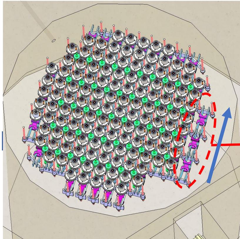
4-Removal of the first row of GRID+support bars+hanging rods
