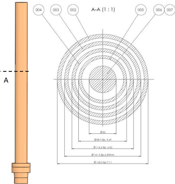
Control Rod Drive Housing and inside parts mock-up (A-A cut)
