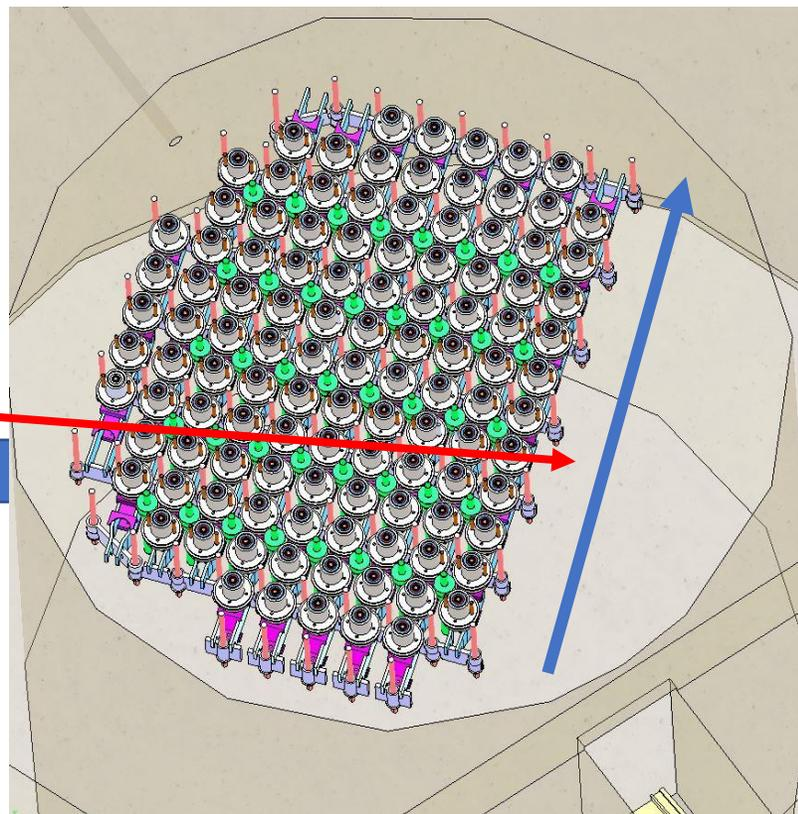
The dismantling operations are repeated until the complete removal of the CRD-H
