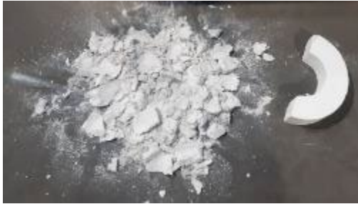
Status of heat insulators (crushed) inside the melter (IR camera (Infrared camera) image)
