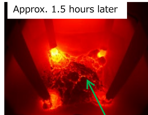
Mostly molten heat insulator (crushed)
