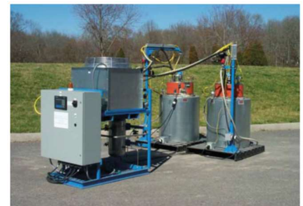
FIG. 19. In-drum drying unit (courtesy of Diversified Technologies Services).
